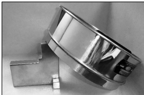
Figure 2-3. Sieve with Tilt Block Set at 30 Degrees.
