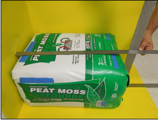
Figure 3-5. The packaging tail on the end of the package can affect this measurement so it has been folded over and taped against the end of the package.
